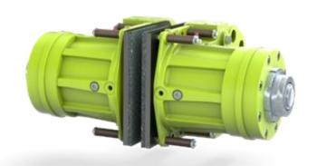
The disc spring pack must be adjusted to compensate for brake lining wear and to maintain full brake capacity. An extension of the brake piston through the adjustment nut gives an easy visual way to tell when adjustment is needed.
